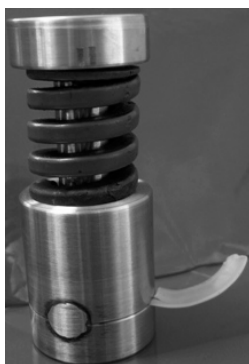
Figure 5. Basic extrusion test of baroplastic PEHA_{0.26} - b - PS_{0.48} - b - PEHA_{0.26} tri-block copolymer (P4) via a custom-made "extruding mold".
