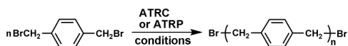
Scheme 5. Synthesis of poly( p -xylylene) by polyrecombination in ATRC or ATRP conditions
